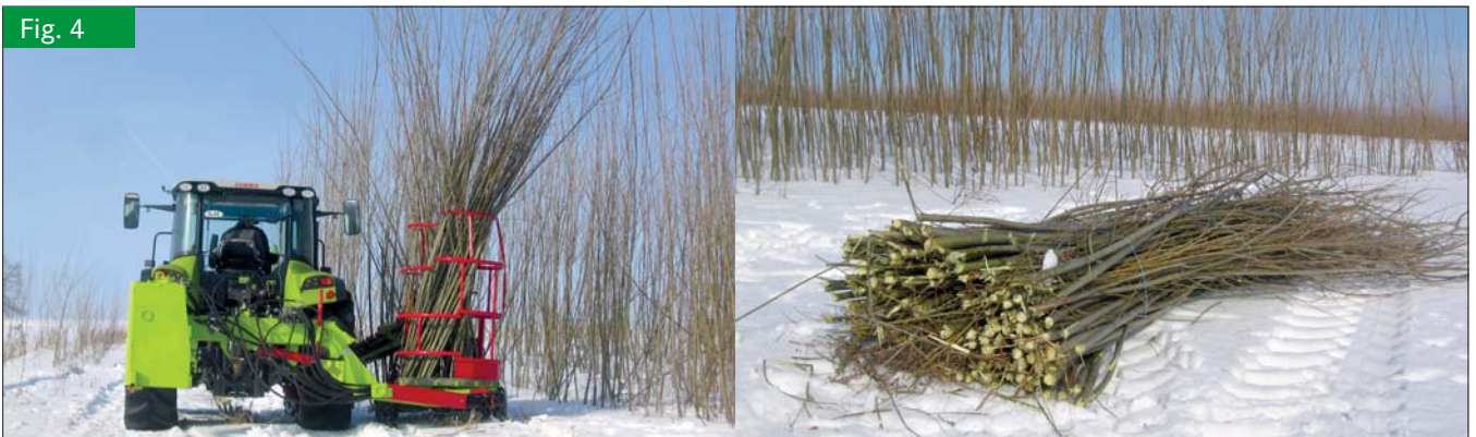
Fig. 4: Prototype, while harvesting bunches (left), mechanical discarded bunch (right). Fotos: Grosa, TU Dresden
