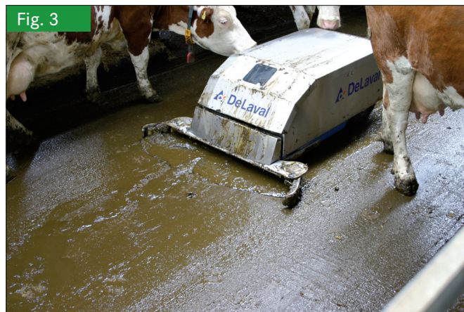
Design of the mobile manure removal machine "slat-cleaning robot" (foto: TUM)
