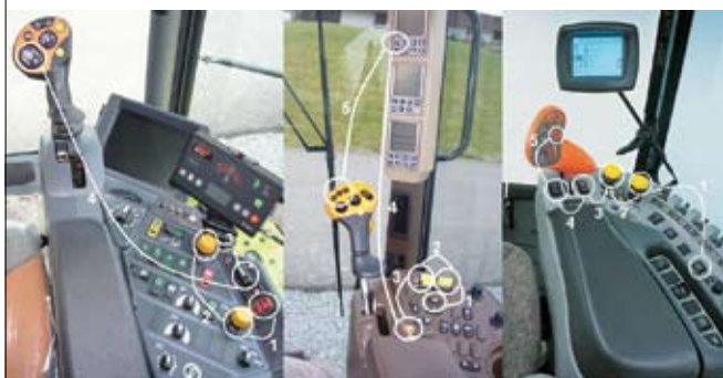
Comparison of the sequence of operation to activate the cutterbar control (left to right: Claas, John Deere, New Holland), acc. [6]
