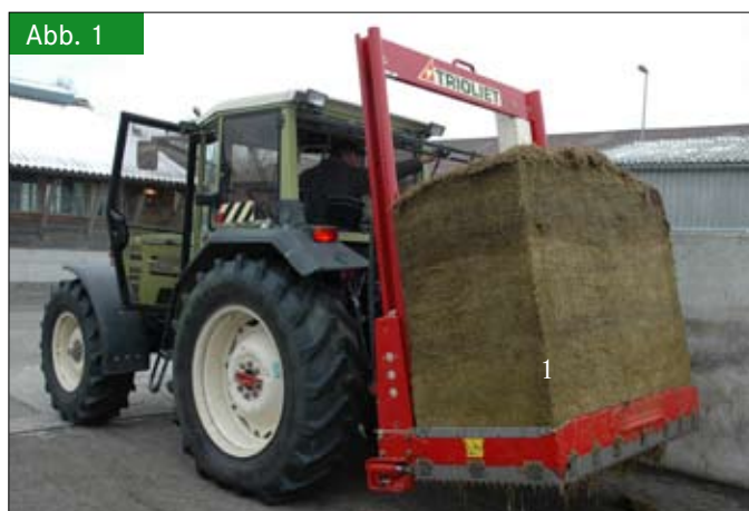
Sampling devices used in the trial: 1 - Silage block cutter; 2 - Drilling cylinder (ART); 3 - Electric silage cutter; 4 - Pioneer™ drilling jig
