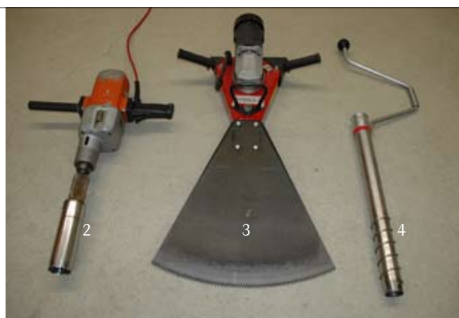
Sampling devices used in the trial: 1 - Silage block cutter; 2 - Drilling cylinder (ART); 3 - Electric silage cutter; 4 - Pioneer™ drilling jig
