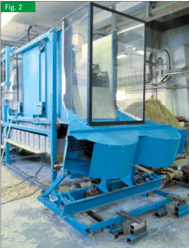
Test rig with feeding equipment
