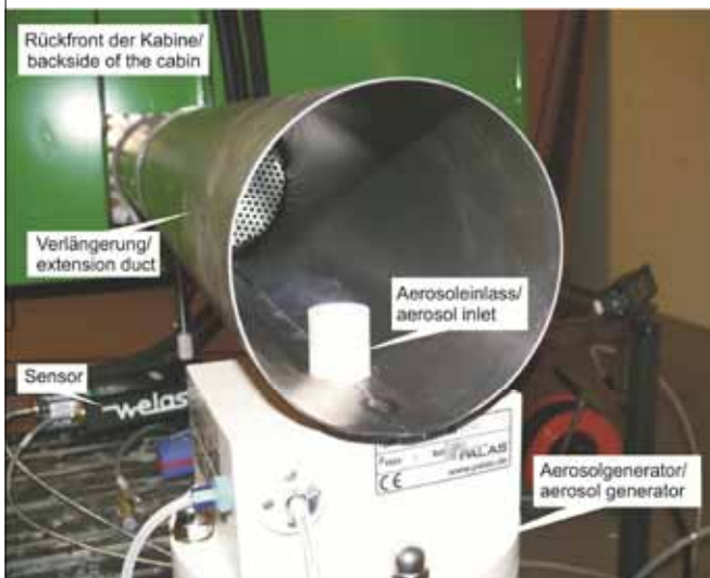
Test-Anordnung zur Messung des Kabinenwirkungsgrades Fig. 7: Test assembly to measure the protection efficiency according to the aerosol test
