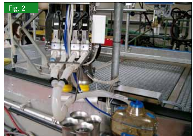
Fig. 2 Prototype of the vacuum control valve in the vacuum control system [8] (Photo: Ströbel)
