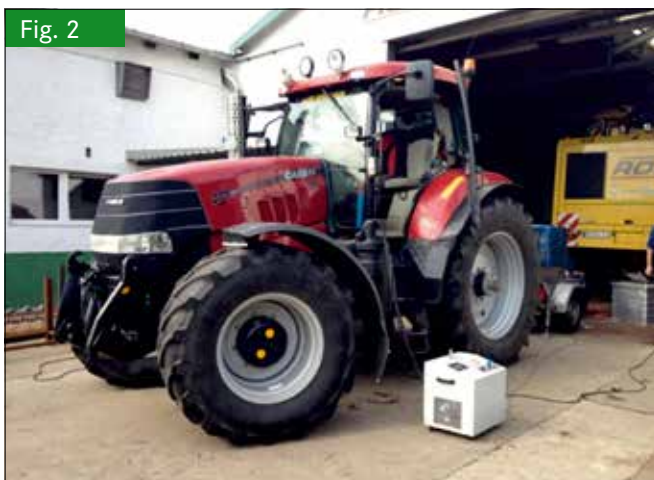
Case Puma CVX 225 during power measurement at the PTO shaft (Photo: Trefflich)
