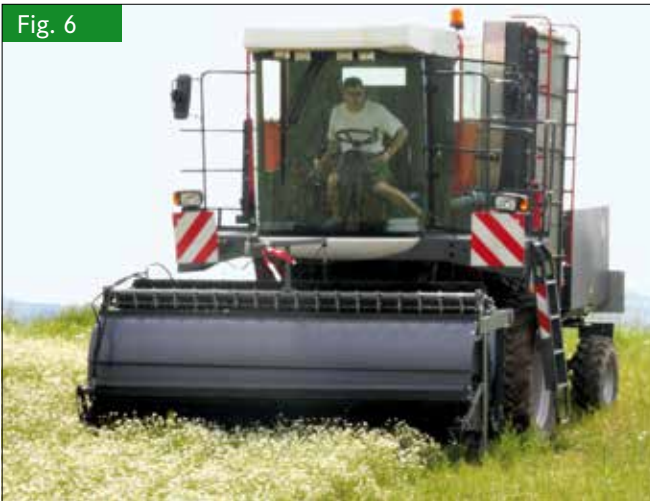
Chamomile harvester KBEM'13 while testing (Photo: ATB)
