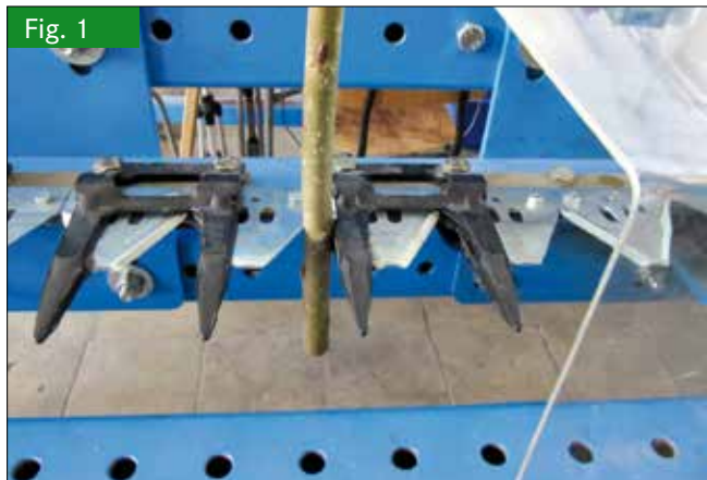
Test stand with cutting distance (left), cutting forces of a cutting bar with fresh poplar rods (right) (Photo: Peschel, TU Dresden)
