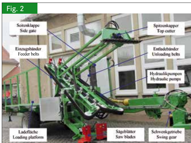
ROD Picker prototype (Photo: Peschel, TU Dresden)
