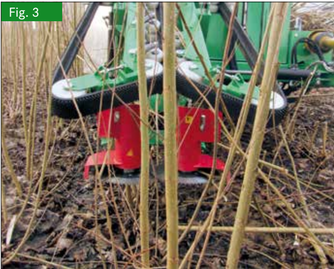
Saw blades and feeder belts (left), unloaded poplar rods (right) (Photos: Peschel, TU Dresden)
