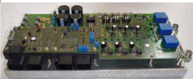
1200V-250A-IGBT water cooled high power inverter
