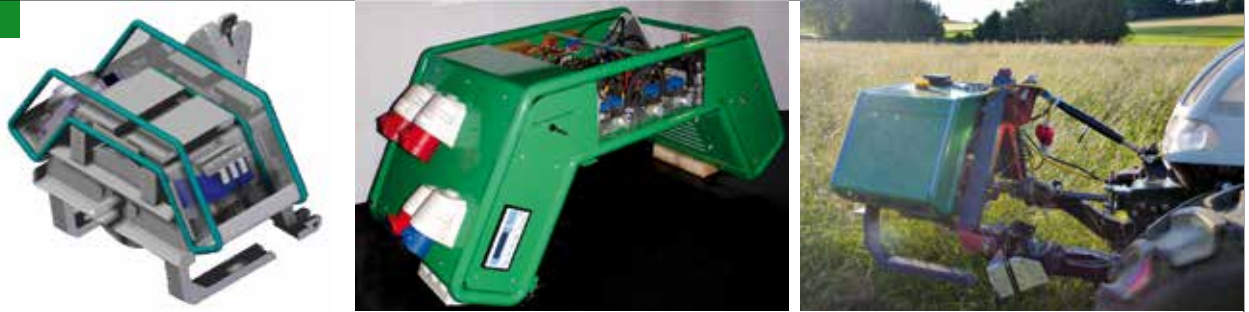
3-D draft of the PTO generator (a), picture of the power pack, half open (b), PTO generator in the field (c)
