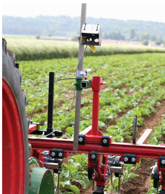
Figure 2: Camera guided hoe and image analysis system to recognize the crop rows
