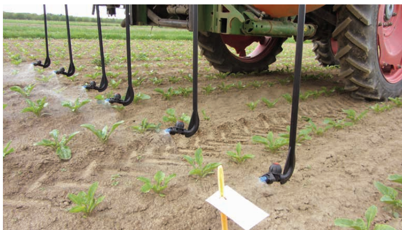
Figure 1: Dropleg for herbicide application at the third date
