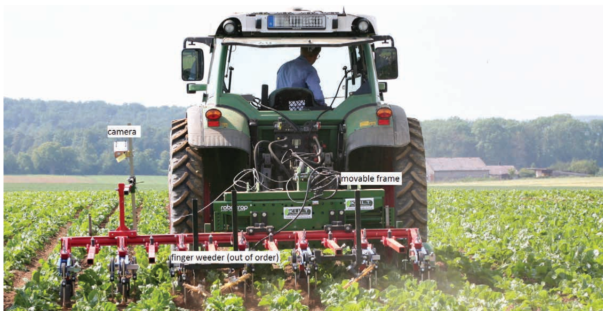
Figure 3: Camera steering system (treatment 3, without finger weeders) to automatically guide the hoe close to sugar beet rows
