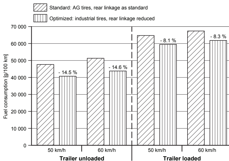
Figure 3: comparative presentation of fuel consumption of standard version and version optimized on road transportation
