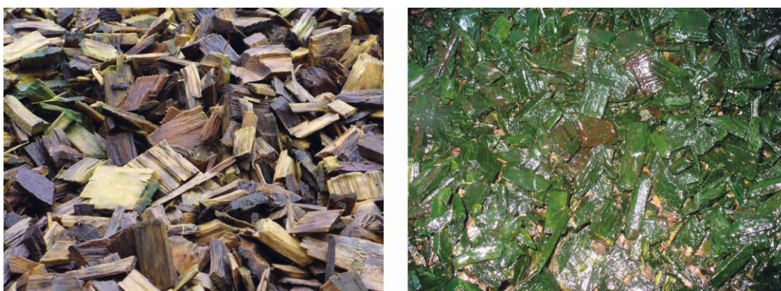
Figure 10: Algae growth on the wood chips layer by nitrogen accumulation
