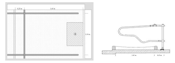
Figure 2: Schematic drawing of the chambers position in the cubicle (left); Lateral view of the cubicle (right, adapted from Sulzberger OHG)
