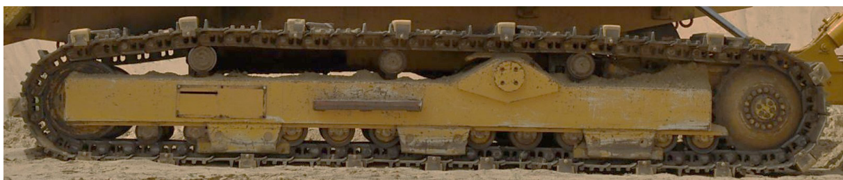
Figure 2 : Lateral view of the track undercarriage – (© TU Dresden, Chair of Agricultural Systems and Technology )
