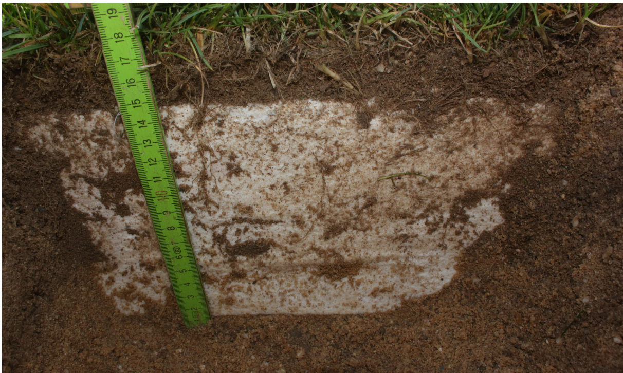
Figure 3: Incorporated nonwoven connecting rootzone layer and drainage layer in one of the test plots. (© B. Stürmer-Stephan)
