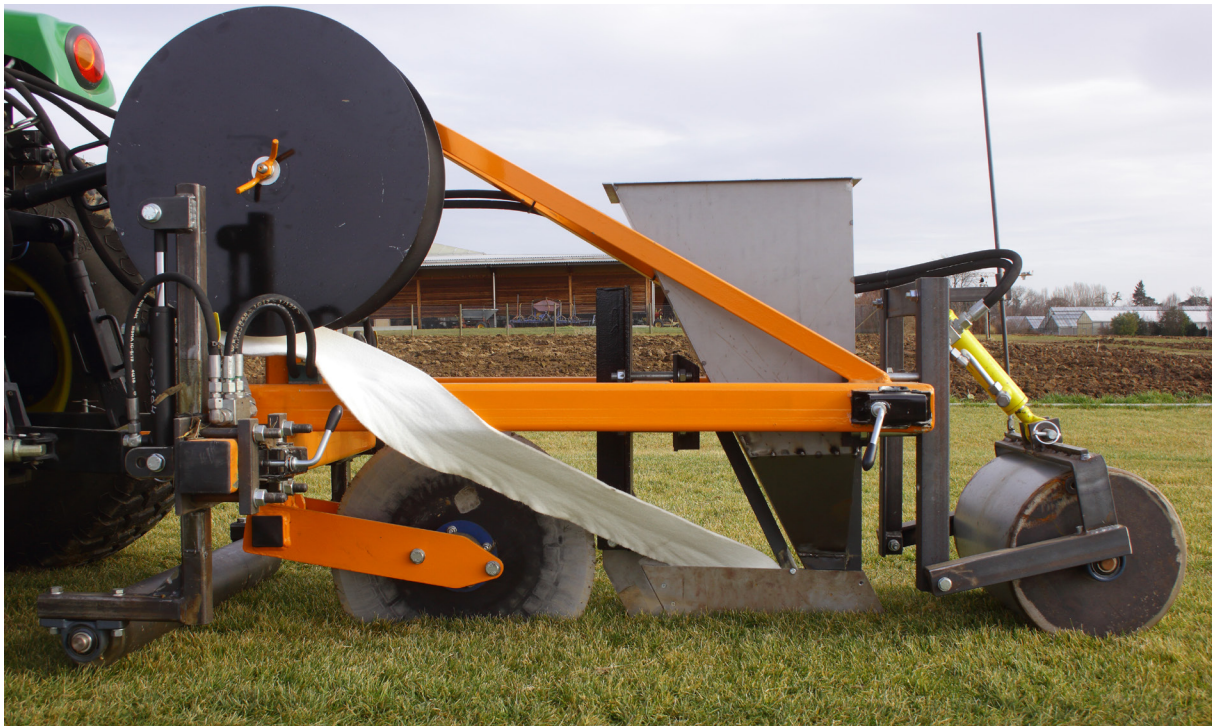
Figure 5. The developed device incorporates a 150 mm height nonwoven in a depth of 170 mm on one of the test plots. The box above the coulter can be used for testing the incorporation of additional sand, but this feature is not investigated within this work. (© B. Stürmer-Stephan)
