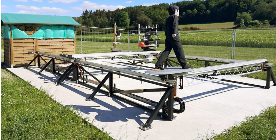
Figure 2: The project “Agro-Safety” used the new test target on a dynamic test stand in a long-term test for 365 days a year and 24 hours a day in continuous outdoor use and different environments (© C. Meltebrink)
