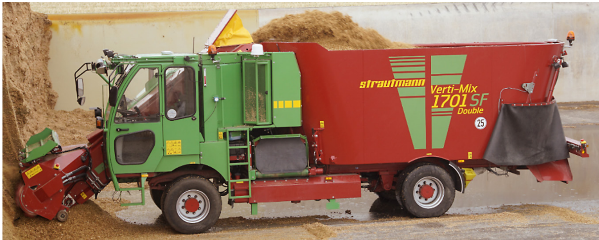
Figure 1: The autonomous feeding mixer “Verti-Q” in a typical working environment (© B. Strautmann & Söhne GmbH u. Co. KG)
